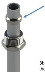
3a. Slide the lock nut and the olive on to the drop tube.
