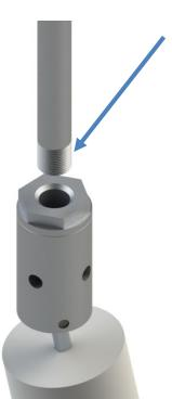
2a. Apply Bondloc B542 (or equivalent) to the thread on the tube.
