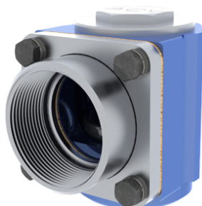
RIS-FLANGE2-SO-SUCTION-R2-MK2 2" female threaded base module for use on threaded tank lid ports.
